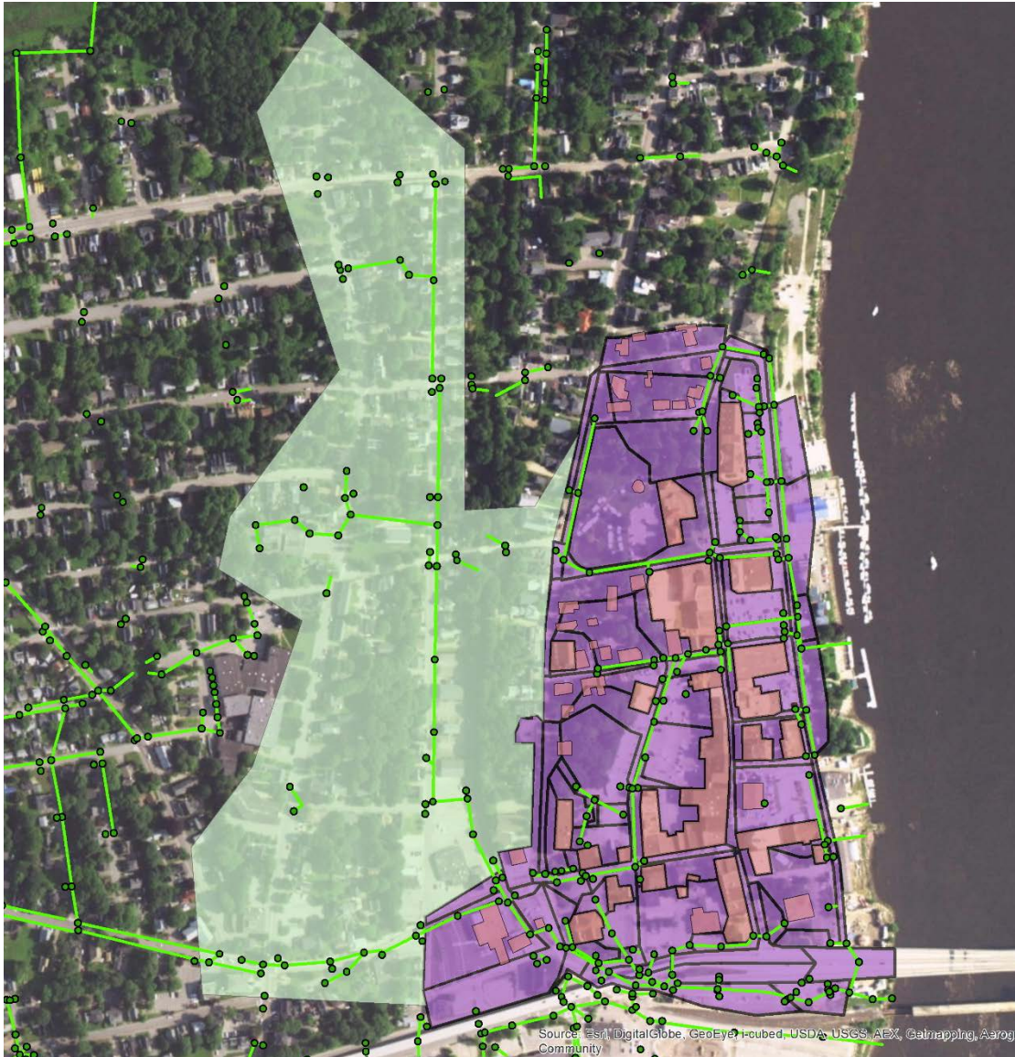
Figure 2-7: City of Bath Downtown Stormwater Study Subcatchment Delineation with Storm Drain Network
