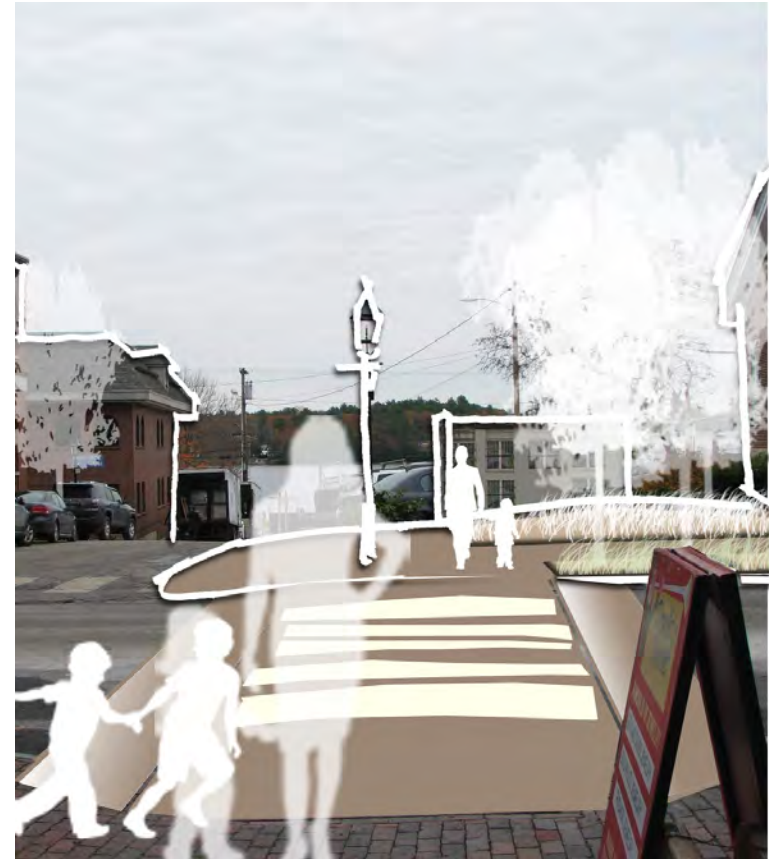
An elevated crosswalk, rain gardens and other detention areas, along with the reconfiguration of the existing diagonal parking on the south side of Broad Street will transform this connector into the main gateway to the waterfront.
